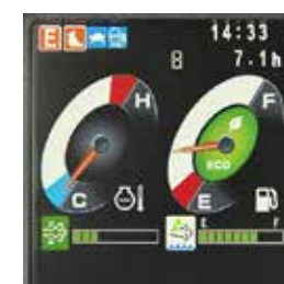
PM accumulation/DEF level
