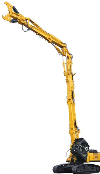
Photo Caption 1: The new KOBELCO SK400D and SK550D building demolition machines feature a 30-degree tilting cab.
