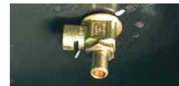
Engine oil quick-drain valve can be turned without, special tools.
