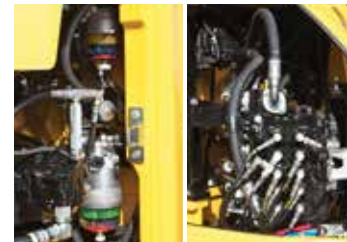
Fuel water separator/Fuel filter/Control valve
