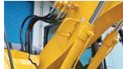
Handhold The handrail on the boom side allows easy access to the top of the machinery deck.
