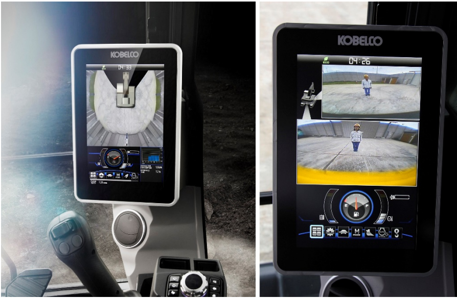
Photo Caption 2: The KOBELCO SK130LC-11 features a new 10-inch color monitor with a split-screen display function to customize operator viewing needs.
