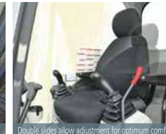
Double slides allow adjustment for optimum comfort
