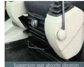
Suspension seat absorbs vibration
