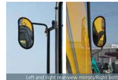
Left and right rear-view mirrors/Right bottom clearance mirror
