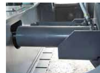
Crawler extension/retraction mechanism guard Hydraulic cylinders are protected from debris. [on SK400DLC and SK550DLC]
