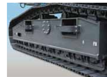
Full track guides* Crawler de-tracking is prevented even on roughest ground littered with demolition rubble.
