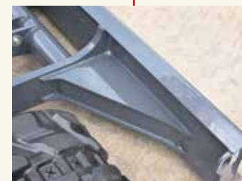
Dozer Box construction dozer supports provide greater strength.
