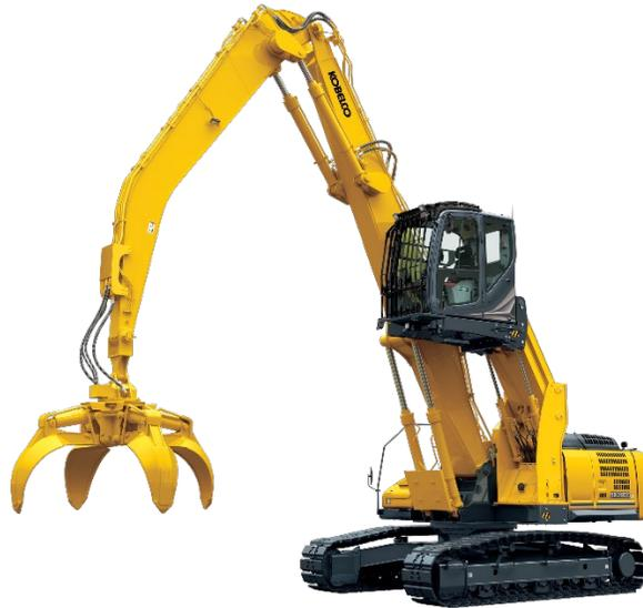
Picture 2: The new SK260DLC-11 Material Handler features a bent boom and a 2-pin linkage-type arm, allowing for both precise movement control and powerful lifting.
