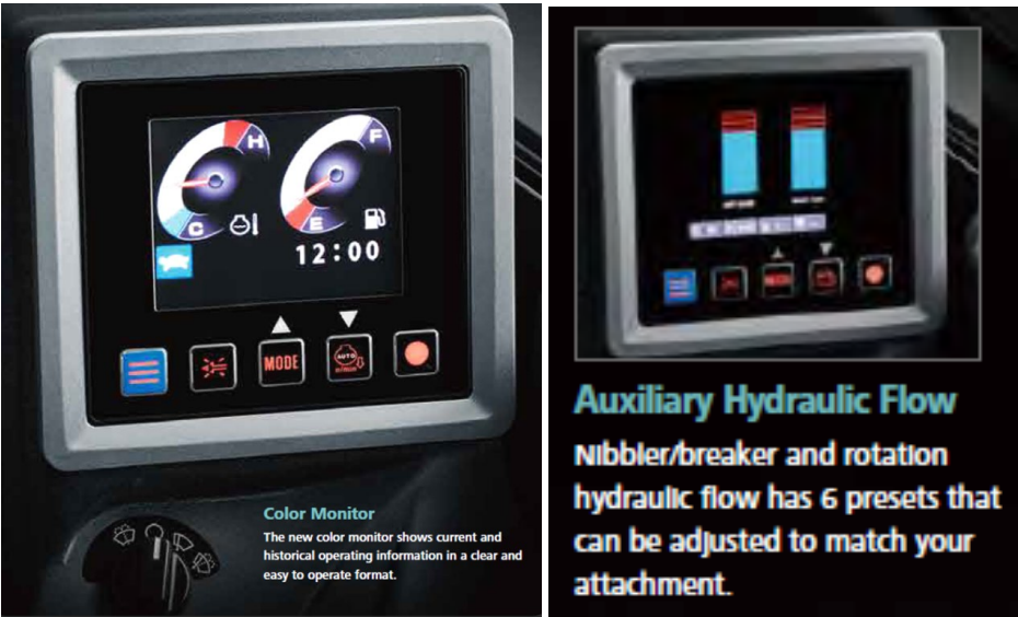
Photo Caption 2: The KOBELCO SK55SRX-7 features a new color monitor with in-cab auxiliary flow adjustment and machine operation/maintenance history.
